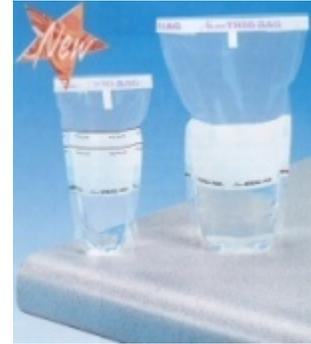
Specially designed for sampling chlorinated water, the Thio-Bag is economical and convenient to use. This single service, sterilized, lightweight, unbreakable container is always ready for immediate use.
